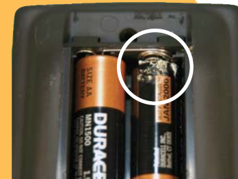
Corrosion you CAN see
