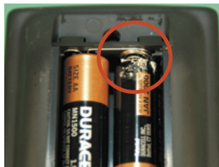
Corrosion you CAN see
